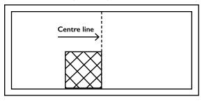
Work out how many panels you would lay across the room. Ensure you do not end up with an edge panel less than 60mm wide. If this is the case, align the centre panel to the alternative, either the centre or the edge.
