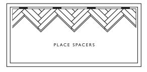
**12.** Continue to install the rest of the area, working from side to side across the room in alternate batches of left-hand and right-hand pieces. Frequently check that the pattern aligns with the installation line
