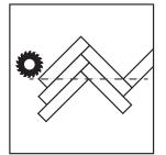
6. Place the back edge against the end wall of the room, with the click groove side facing outwards, and align the front corner with the installation line. START WALL
