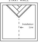
7. Measure the total width of the room and calculate how many starting triangles will be needed. Form and place these triangles as before. Measure the remaining spaces at both sides of the room and form the extra triangles to fill the spaces.
