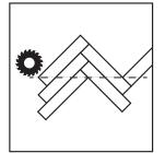
6. Place the back edge against the end wall of the room, with the click groove side facing outwards, and align the front corner with the installation line. START WALL
