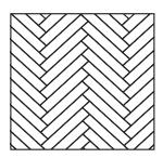
**I.** Identify the left-hand and right-hand planks before installation. The herringbone planks are designed to be laid working from side to side across the room in alternate batches of left-hand and right-hand pieces.
