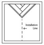
**7.** Measure the total width of the room and calculate how many starting triangles will be needed. Form and place these triangles as before. Measure the remaining spaces at both sides of the room and form the extra triangles to fill the spaces.
