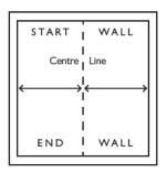
3. Measure 45mm to the right of the centre line and mark the installation line.
