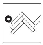
**6**. Place the back edge against the end wall of the room, with the click groove side facing outwards, and align the front corner with the installation line.
