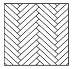
1. Identify the left-hand and right-hand planks before installation. The herringbone planks are designed to be laid working from side to side across the room in alternate batches of left-hand and right-hand pieces.
