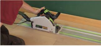
5. Then, test the cut for size using a piece of the design strip.
